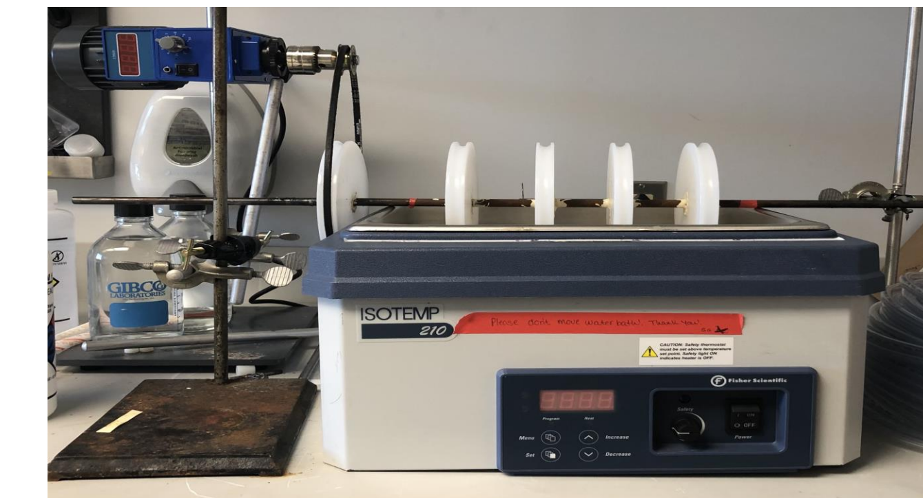
Fig. 3 Chandler Loop Apparatus: Photograph showing the design of the Chandler Loop Apparatus. This will be used to mimic physiological conditions of cell attachment to a biomaterial.
