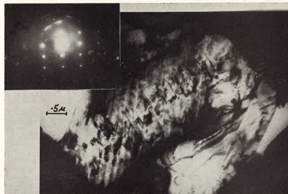
Fig. 15. Electron micrograph and superimposed selected area electron diffraction pattern of a typical fracture trough in a stainless steel foil.
