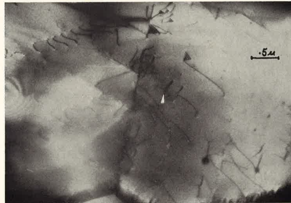
Fig. 13. Electron micrograph showing a compressed area in a stainless steel foil. Dislocations have been pinned at one surface, and have elongated in the slip planes under the action of the applied stress.
