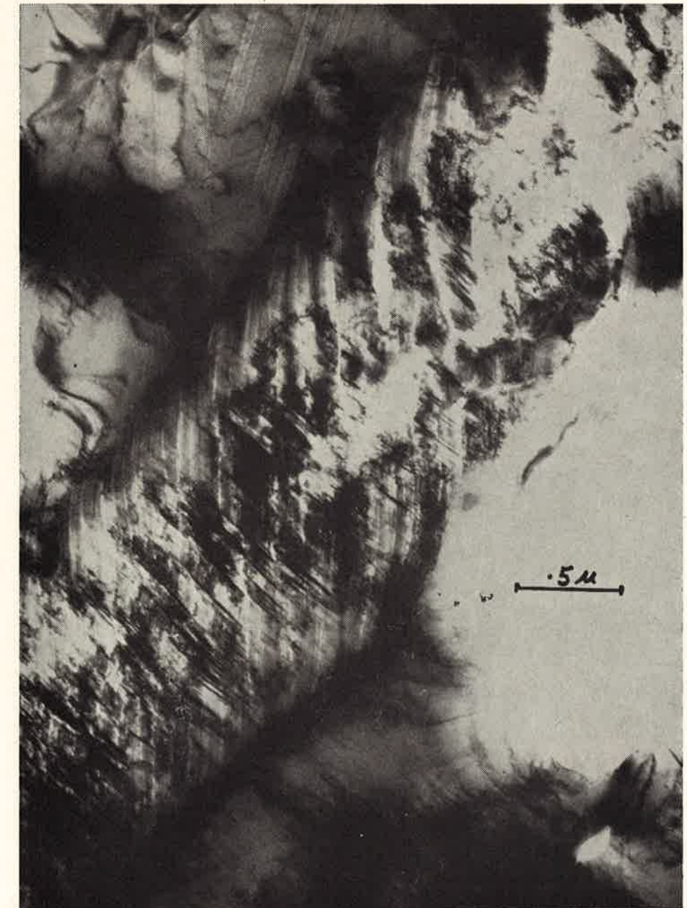
Fig. 14. Electron micrograph of a fracture trough in a stainless steel foil produced by rolling contact stresses. (rolling steel ball)
