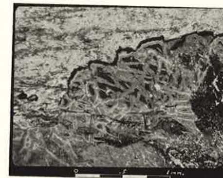
Fig. 3. Part of a large pod of altered cordierite, exhibiting anastomosing structure. Pod lies in pure, fine-grained talc. Crossed polars.
