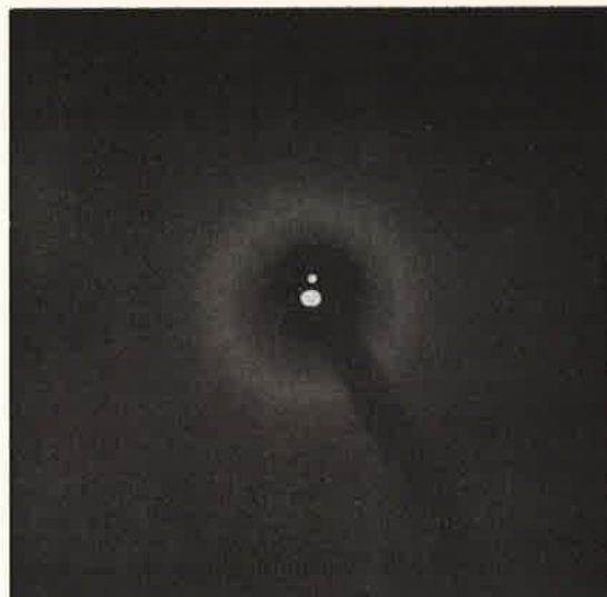
Figure 12. X-ray Diffraction Pattern of the Low Boiling Fraction of the Ethyl Ester of Undistilled Naphthenic Acid at -152^{\circ}\text{C} .
