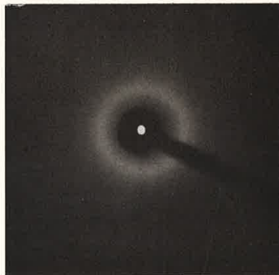
Figure 13. X-ray Diffraction Pattern of the Low Boiling Fraction of the Ethyl Ester of Undistilled Naphthenic Acid at -132.5^{\circ}\text{C} .
