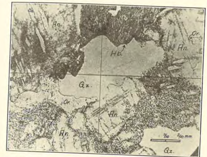
FIG. 2. Photomicrograph showing andesine (An), hornblende (Hb) and orthoclase (Or) being replaced by quartz (Qz). Orthoclase had previously replaced andesine along the margins of grains as shown in the grain at the upper left. Note the intense sericitization of this grain and also the one at the right between the two quartz areas.
