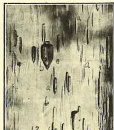
12 x300 Willemite (1120), Etched by Sodium Hydroxide Fusion
