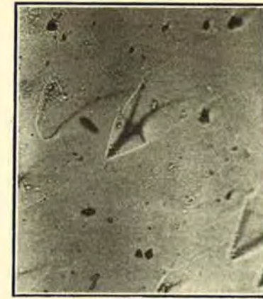
8 x300 Willemite (1120), Etched by Sulfuric Acid
