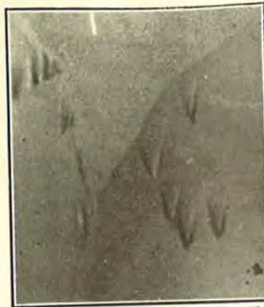
4 x180 Calcite (2131), Etched by Citric Acid
