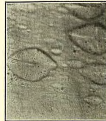
9 x300 Calcite (1120), Etched by Concen- trated Citric Acid
