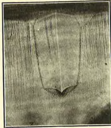
3 x30 Calcite (1011), Etched by Citric Acid
